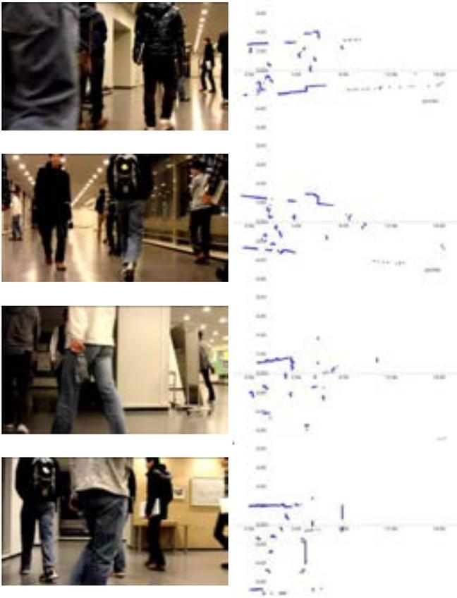
Fig. 12. Snapshots of images obtained from digital camera (left column) and SICK LMS100 (right column) installed in the robot.
