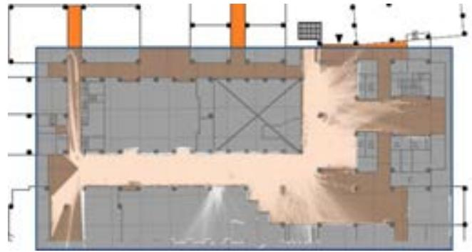
Fig. 14. The occupancy grid map obtained by the open SLAM software *MRPT* and the proposed method. We overlay the floor plan of this building to evaluate the accuracy.
