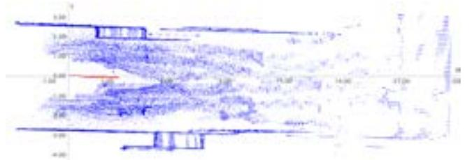
Fig. 6. The map estimated by the  $L_2$ -norm minimization with 30 percent threshold. The red line indicates robot's displacement and the blue points indicate measured points on the global coordinates. Since the robot is fixed, the red line should not appear. Since the blue points on the outer boundary corresponds to the wall of the building (Fig. 5 (c)), they should not be blurred.
