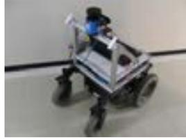
(a) LIDAR: SICK LMS100 (b) Mobile robot: EMC-230
