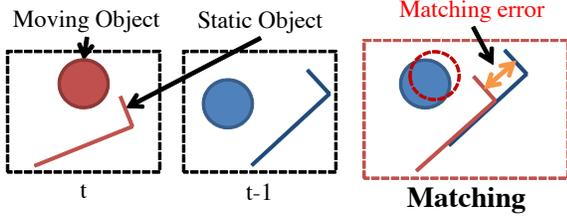
Fig. 1. Erroneous estimation of displacement due to dynamic environment. The circular object moves rightward from time  $t-1$  (middle) to time  $t$  (left), while the L-shape object is fixed. Alignment only using the L-shape object outputs the correct displacement. But the prior scan-matching methods diffuse matching errors uniformly in the space, resulting in erroneously estimating the displacement.
