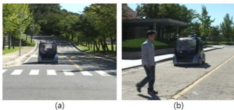
Figure 11. (a) ESTRO stopped in front of stop line for compensation on the intersection, and (b) ESTRO stopped when the pedestrian crossed the road.
